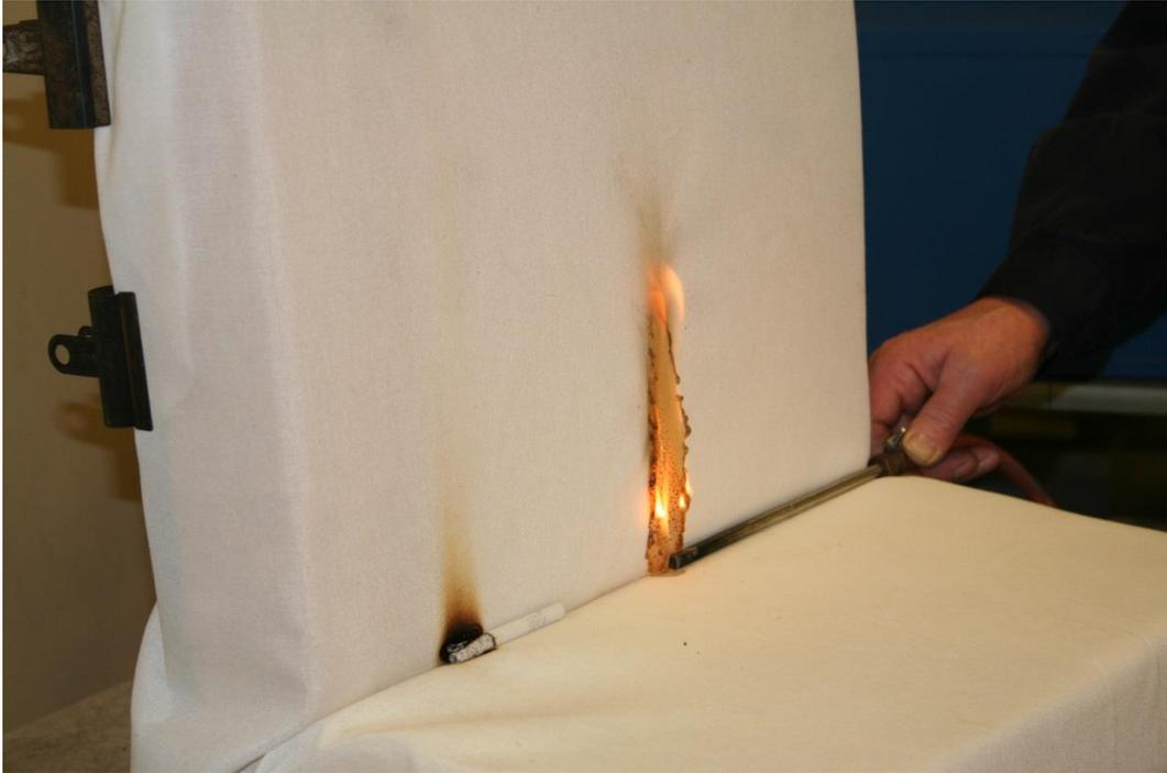
**Figure 7-2** Demonstration – smouldering cigarette and match-flame equivalent on an IMO 2010 FTPC Part 8 upholstery material assembly.
