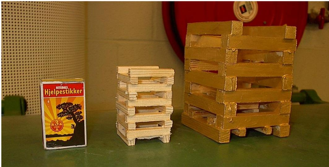
**Figure 7-1** Varying sizes – a small box of matches alongside a wooden crib no. 5 and no. 7.
