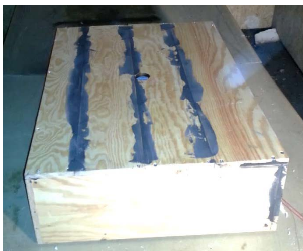
Figure 4-4 Complete setup of source of fire, where the mattress and smouldering fire generator are covered by a crate with a hole to allow fire smoke and gases to escape.
