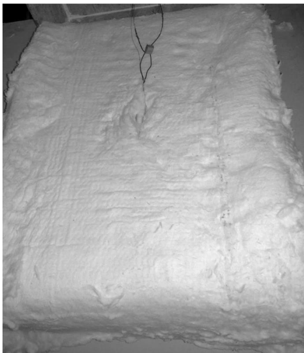
Figure 4-2 Mattress segment packed in ceramic wool with the "smouldering fire generator" inside.
