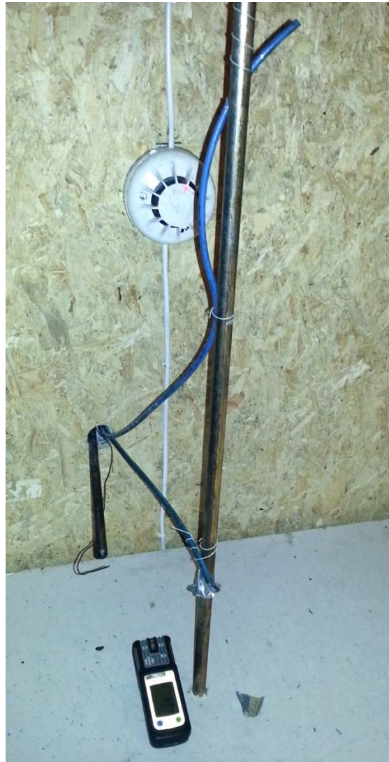
Figure 4-9 Locations of extraction of CO/CO 2 -measurements and FTIR at the head end of bed.
