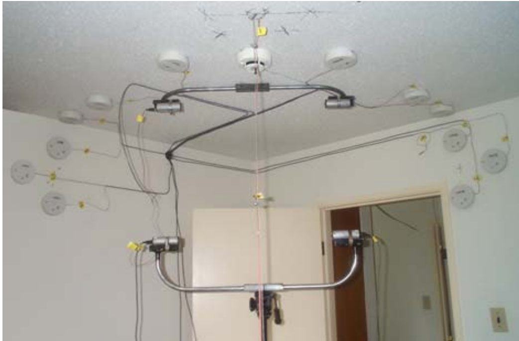
Figure 3-2 From one of the experimental setups examining the effect of dead-air space. Smoke detectors of different brands were installed in different room locations, both inside and outside the zone required in North America. Photo: [5].
